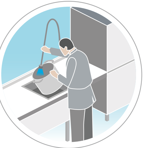
Keeping steam in the dishwasher reduces heat and humidity in dishroom and eliminates the need for a costly vent hood.
